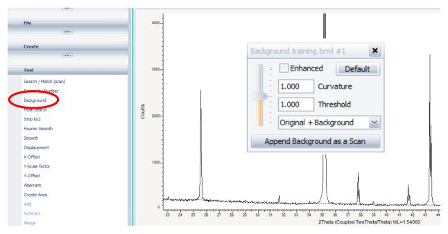
The background is approximated by the dashed line. Adjust the vertical slider to get the best fit. Open the dropdown menu and select 'background subtracted.' Close the dialog box.
