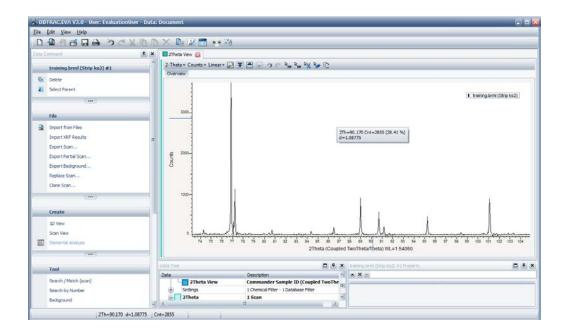
Next, if working with a known sample, determine whether the reference peaks are positioned at the correct 2 theta values. For corundum zero in on the highest peak at 35.149°.
