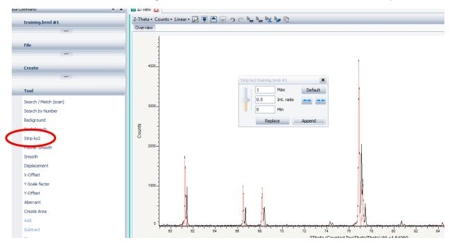
Adjust the slider to get the best fit and select 'Replace'. Use 'Append' if you wish to save the original pattern for later. The modified pattern should then look like:
