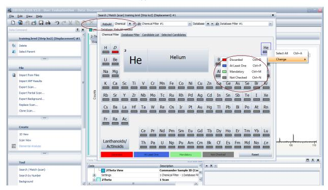
By left-clicking and dragging, blocks of elements can be highlighted at once. Upon assigning the appropriate logic to selected elements, click 'Rebuild' in the upper left hand corner to apply the filter.
