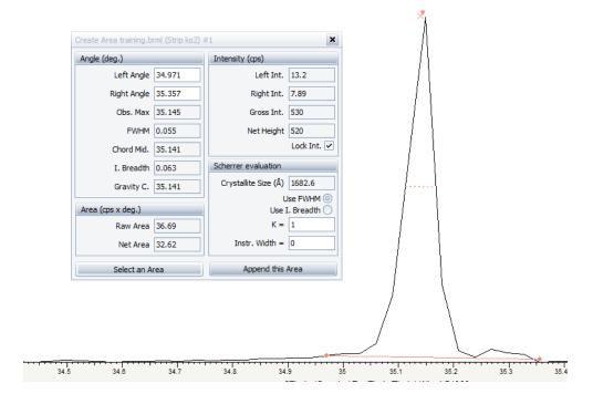
From the box on the left, the Observed max is 35.145. The literature value for this sample is 35.149. The instrument precision is 0.01 degree. The difference between 35.145 and 35.149 is less than 0.01, thus no shifting of the pattern is necessary.
