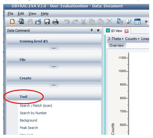
First, the background must be subtracted. Zoom in at a low angle part of the pattern by drawing a rectangle and click Background in the Tool menu.
