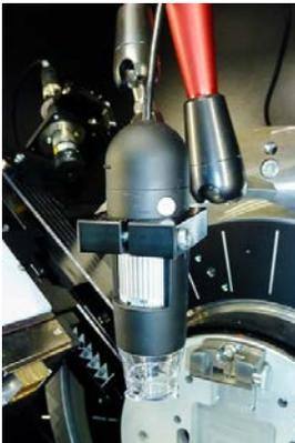
Conventional samples in round sample holders should be placed on the spring plate, the plate goes just beneath the wings, and the spring goes beneath the plate (photo below left). The plate and spring can be removed with two fingers (one on each side of the spring).
